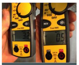
Field test: the current drawn of a refrigeration system before and after a FSE RIDGETech motor retrofit at Boston Market. The current drawn by the system is reduced from 3.2 to 0.5 amps.
